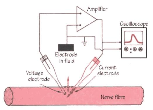
One of these is for the purpose of measuring the voltage of the membrane potential and the other conducts electrical current into and out of the nerve fibre. Current is applied via the current electrode until a rate is reached holding the voltage at steady at -90mV as measured by the voltage electrode.
